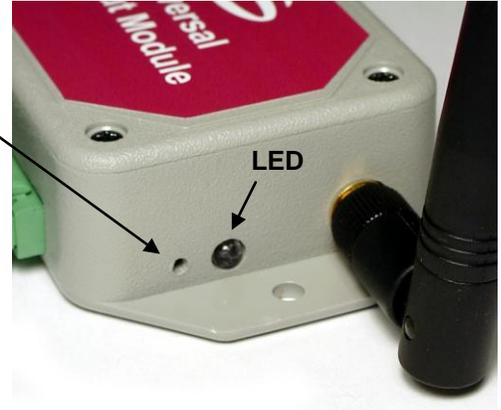
**Application:** Apply the sensor to a surface near the device to which the output is to be connected. Provide power in the form of 12-24 VDC. Note: the UOM can be powered by as little as 8VDC in the case where the analog output is set to the low range (0-5V or 0-20mA.) 12V or higher is required for 0-10V analog output only. The power supply should be capable of providing .2 Amps of current and shares a common ground return with the analog output and counter inputs.
