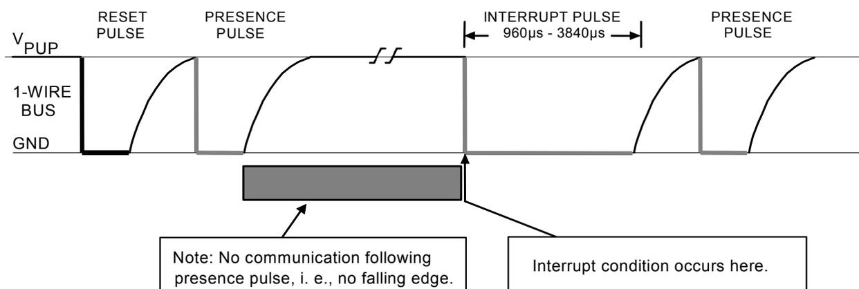
**Figure 13. TYPE 1A INTERRUPT (SPECIAL CASE)**
