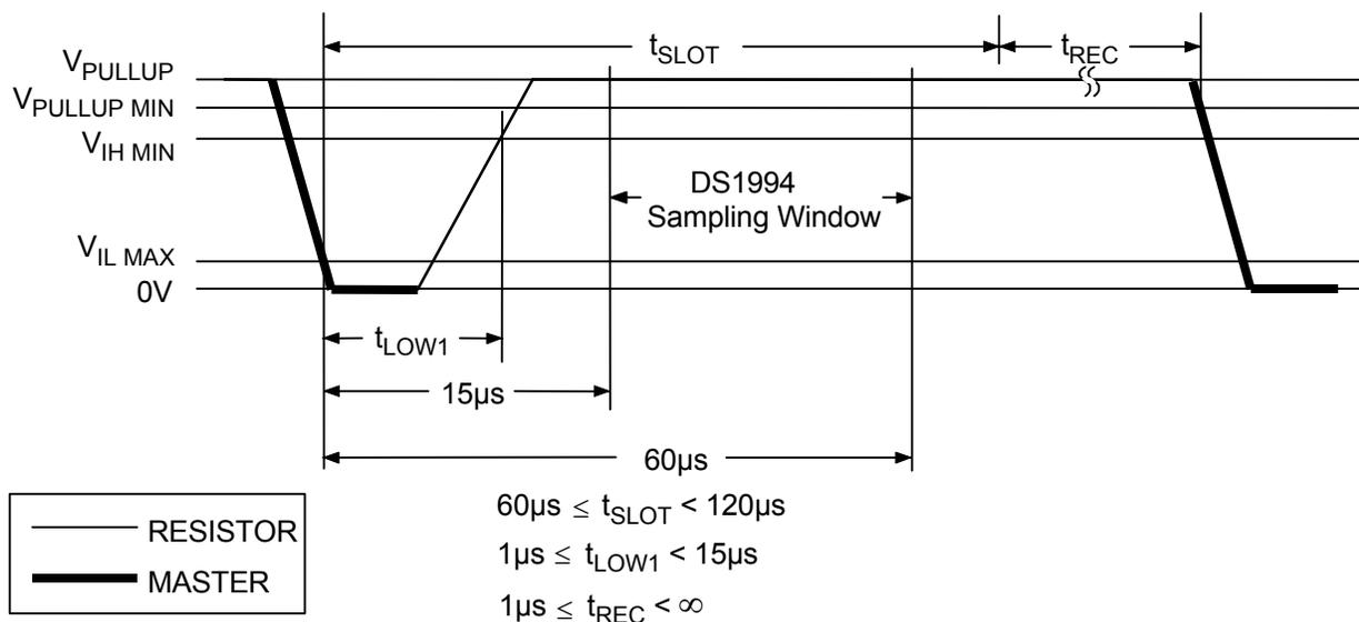
**Figure 11. READ/WRITE TIMING DIAGRAM (continued)****Write-Zero Time Slot**
