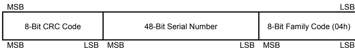
**Figure 3. 1-WIRE CRC CODE**
