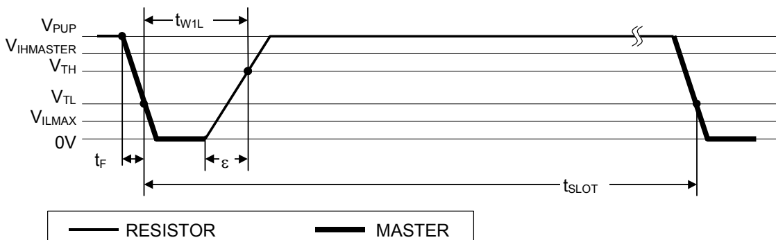
Figure 11. READ/WRITE TIMING DIAGRAM
