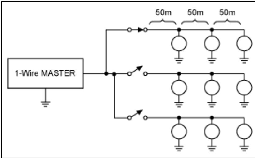
The example above appears like a star topology network with a radius of 150m and a weight of 450m. However, when each switched path is considered individually, the network is actually a linear topology and the weight is only 150m.
