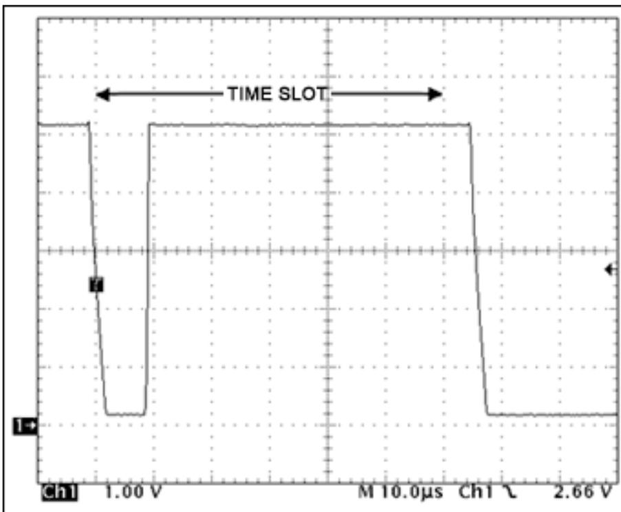
This image shows a Read One or Write One time slot. The master pulls the bus low for about 10µs and then releases it. Note the slew-rate-controlled fall time. The time slot lasts for about 70µs, after which another time slot occurs. Note that the time base is changed to 10µs per division.
