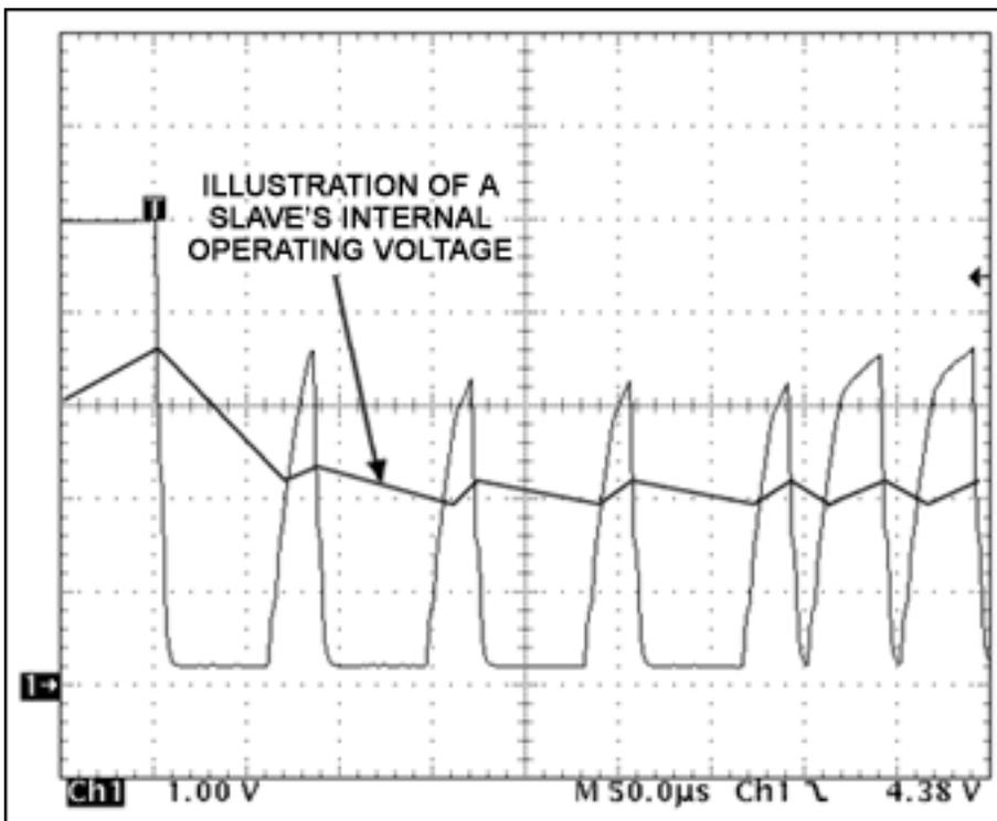
When rise time is slow, the recovery time (the period between time slots) may not be long enough to allow the bus to reach a voltage level sufficient to recharge the slaves. In the image above, the slave's internal operating voltage has become dangerously low. Slaves may reset due to power starvation, especially during long strings of Write Zero time slots.
