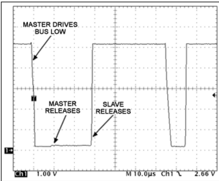
This image shows a Read Zero time slot. The master pulls the bus low for about 10µs and then releases it. However, a slave is returning a zero bit by holding the bus low for a longer time. The slave's time base can vary between 15µs and 60µs.
