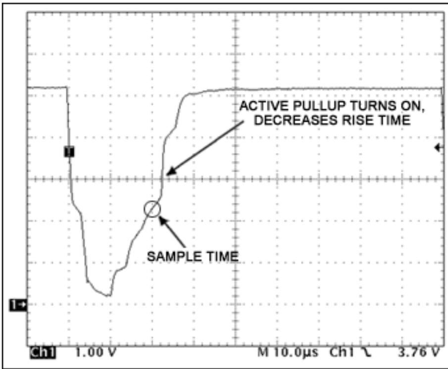
A more advanced network bus driver uses impedance matching and active pullup to overcome the added weight of the long network and slave devices. This waveform shows a Read One or Write One time slot and the action of the active pullup.
