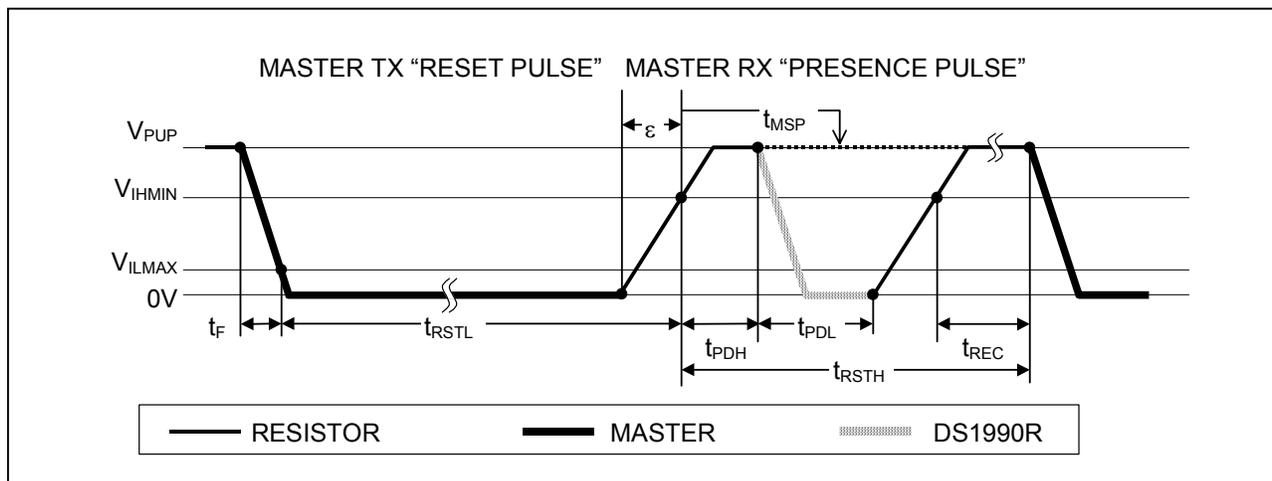
After the bus master has released the line it goes into receive mode (RX). Now the 1-Wire bus is pulled to  $V_{PUP}$  via the pullup resistor or, in case of a DS2480B driver, by active circuitry. When the  $V_{IHMIN}$  is crossed, the DS1990R waits for  $t_{PDH}$  and then transmits a Presence Pulse by pulling the line low for  $t_{PDL}$ . To detect a presence pulse, the master must test the logical state of the 1-Wire line at  $t_{MSP}$ .
